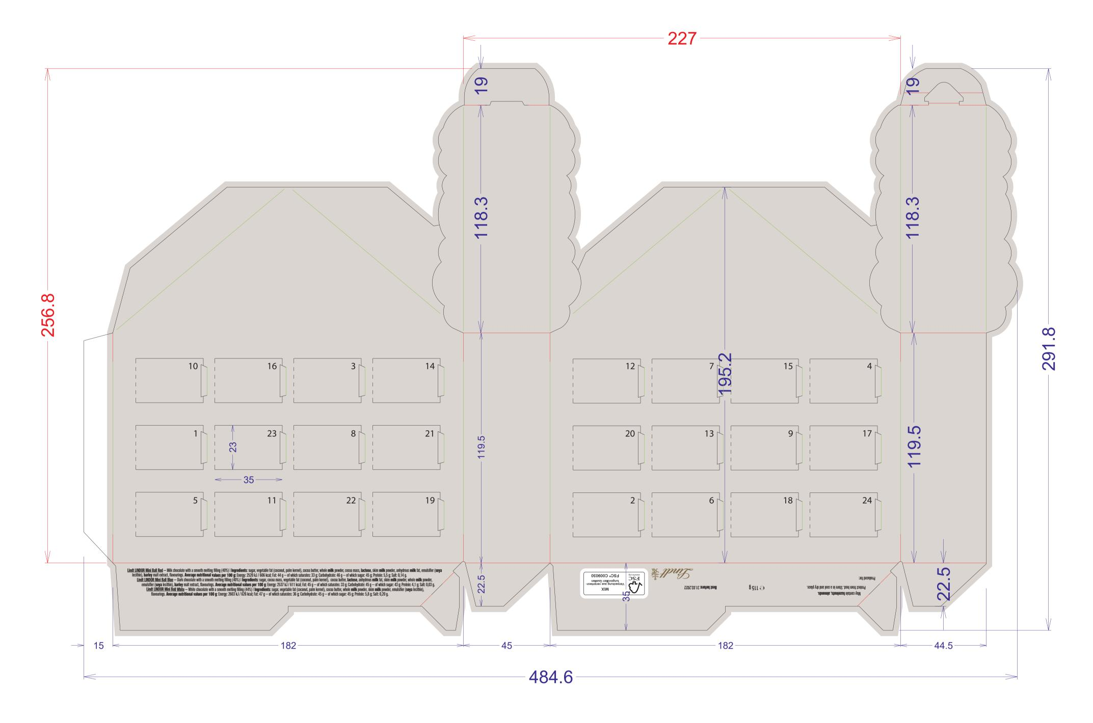
Distance between logos or text and cutting edges should be at least 2mm! Add at least 3mm cut-off!
